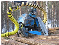
The boom of a cut-to-length harvester with attached chainsaw cutting Pinus sylvestris
